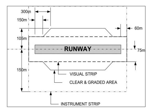
Figure 5-1 Graded portion of a runway strip
