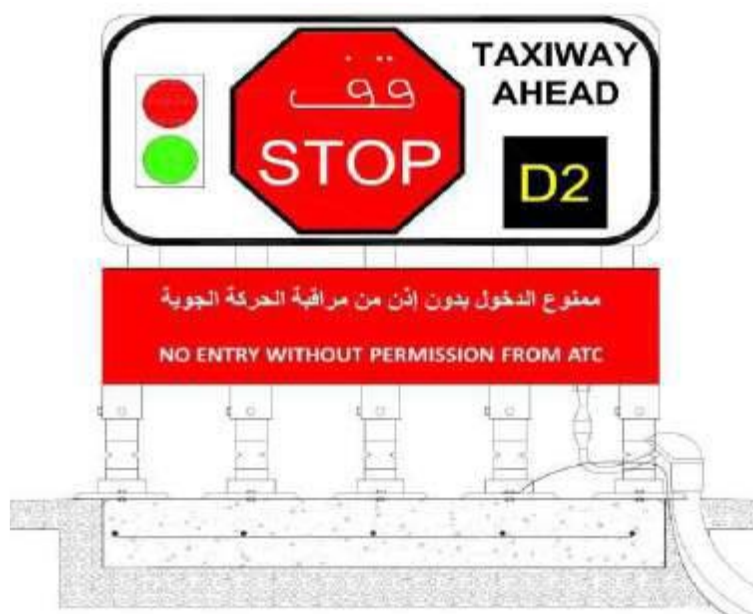
Figure 5-31. Road Holding Position Sign and Lights
