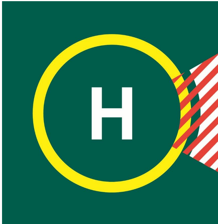
Figure 6: Example of prohibited landing heading marking
